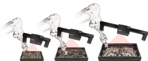
**Available in various sizes, the new 3D solutions allow for safe gripping of small parts as well as large and even bulky units.**
