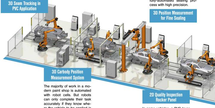
dern paint shop is automated with robot cells. But robots can only complete their task accurately if they know where the vehicle to be applied is located. Because no mechanical vehicle centering units are used in the paint shop or the seam sealing area, contactless, optical 3D position detection of complete bodies is employed here.
