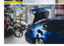
Wheel assembly is usually a manual process still today, and is a monotonous and very physically demanding task. The assembly lines are designed for continuous or stop-andgo operation and can now be completed by robots period at end of sentence thanks to the support of a highly-flexible 3D robot guidance system. The sensors determine the 3D position and orientation of the brake disk and holes or bolts on it, so that the wheel can be installed reliably.
