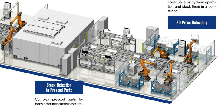
Complex pressed parts for body production may have process or material defects that can lead to production problems as body construction progresses. These defects need to be detected earlier so that the affected pressed parts can be discharged. This is done with a machine vision system, equipped with four line cameras, that inspect all pressed parts in production in motion.
