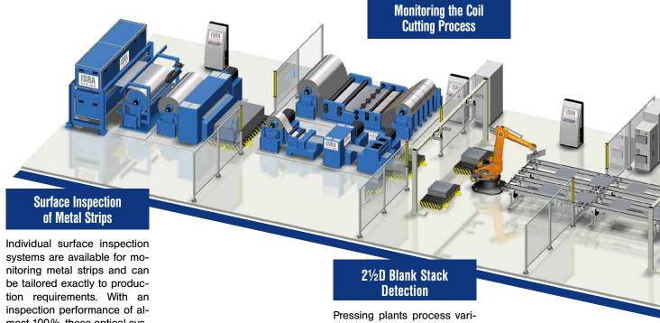
most 100%, these optical systems ensure that only the most immaculate material is turned into components for body production in the pressing plant.
