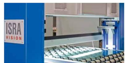
**P<sup>2</sup>-COLOR** reliably monitors the color of coatings and helps secure a consistent, standardized optical impression of the glass plates while saving resources.
