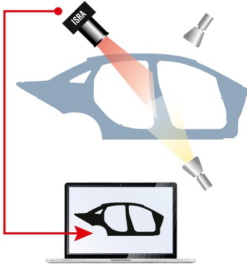
The shape of each individual object to be inspected is captured by transmission.
